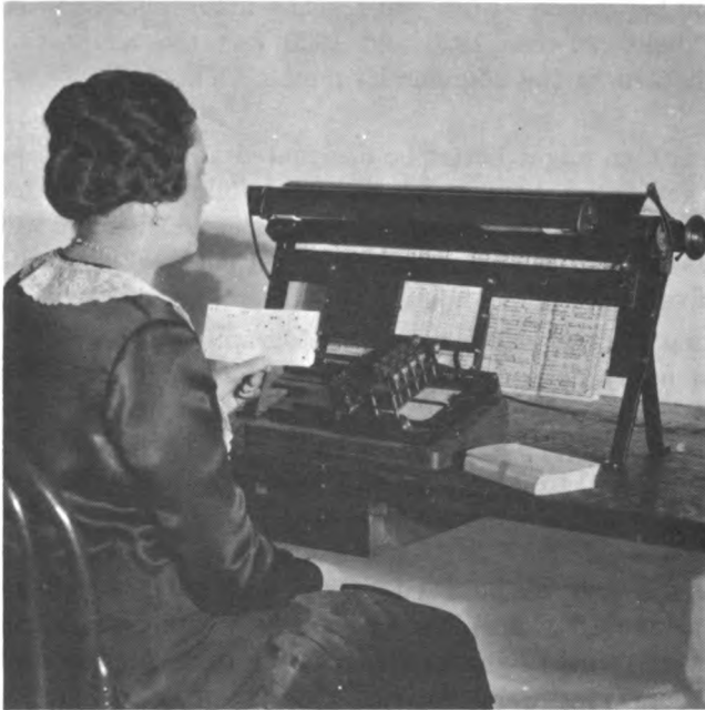
FIGURE 49.—Commercial punch with guide card. The guide card in the machine, as illustrated, is the card used in the second stage of development, as outlined below, as witness the three columns (for occupation) at the end of the card. The schedule in the schedule holder is one of the 1920 schedules which were used in experimental work—and in the testing of the several stages of the adaptation.
